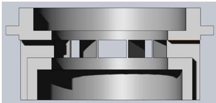
Figure 3.8: Section view of the final version of the strainer insert.
